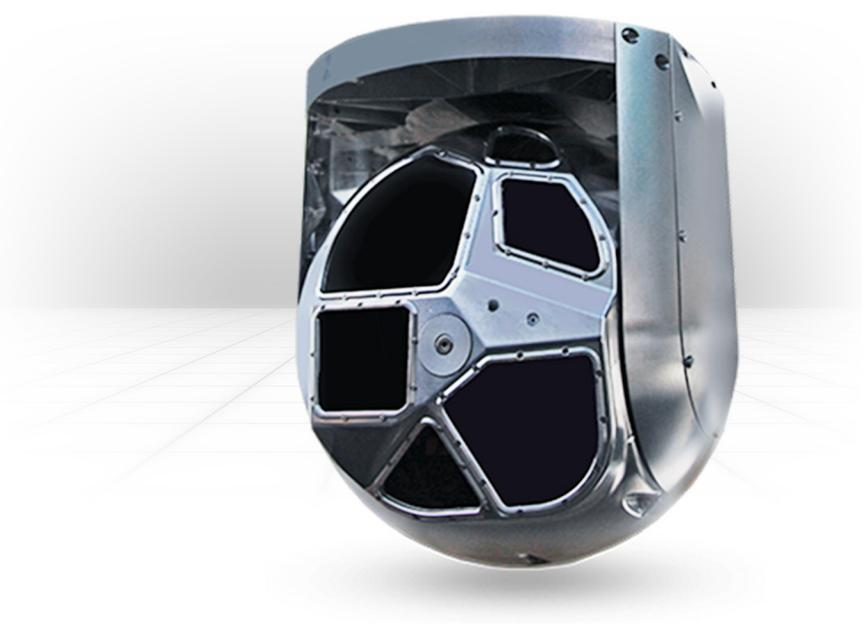
Developed for TUAS, the CM234 combines seven sensors in a compact, four-axis payload. The system includes two HD EO sensors, one MWIR sensor, one SWIR sensor, a laser range finder, a laser target designator, and a laser pointer all in one lightweight package. All together, the CM234 system demonstrates a cutting-edge surveillance solution for UAS, lightweight aircraft, and other platforms.
