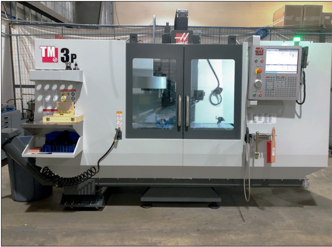
This milling center is 57.8" in length by 14.5' in width, and its 3D graphic GibbsCAM programming ensures automatic precision. Accuracy is \pm 0.0004 " positioning, and \pm 0.0002 " repeatable.
