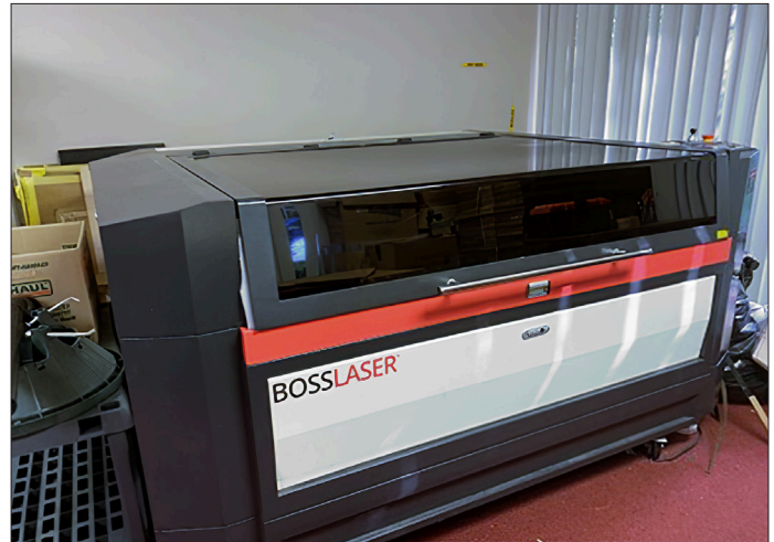
Our laser cutter/etcher cuts, etches, and marks a variety of sheet materials using a focused laser.
