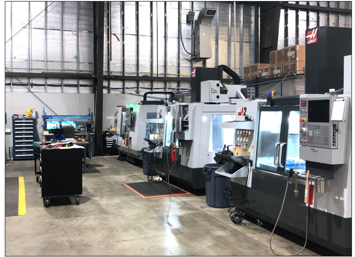
Our FV2 3 Axis milling centers are 36" in length by 14" in width, and also feature 3D graphic GibbsCAM programming. Accuracy is \pm 0.0002 " positioning and \pm 0.0004 " repeatable.
