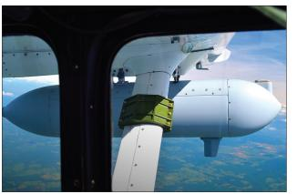
CACI designed and built the Airborne SIGINT pod in support of a U.S. Army program to demonstrate the transition of a ground-based sensor to an airborne platform.
